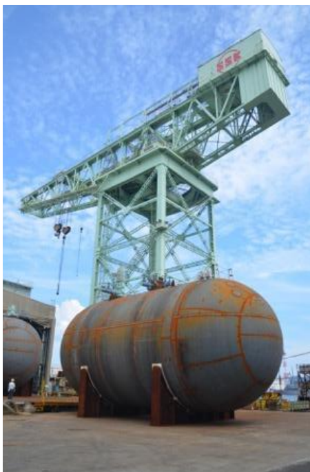
Figures 21 and 22: The Sasebo Crane in 2015 lifting pre-fabricated tanks, and its sister crane at the Walker Yard in Newcastle upon Tyne, England, experiencing a new life after being uprated to serve the UK’s offshore oil and gas industry. (Images: Miles Oglethorpe)
